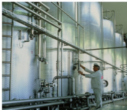
Figure 1.37 Lactose free milk is produced industrially by pouring milk through a column containing the enzyme lactase immobilised in gel beads. The lactase catalyses the hydrolysis of the lactose. Syrup which is used in the food industry is produced in the same way from whey waste from cheese-making.
